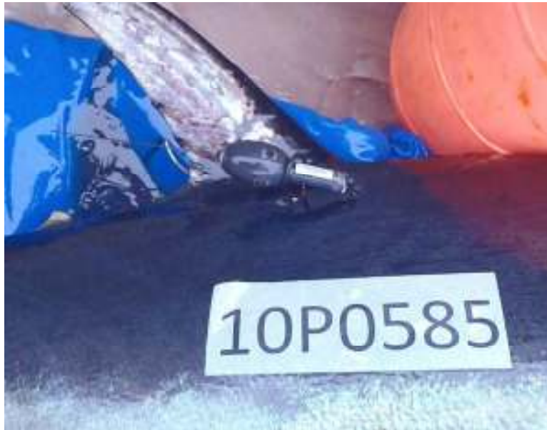
Fig. 1. Photograph showing deployment of a miniPAT tag that is secured externally to an Atlantic bluefin tuna using a two-point attachment technique.
